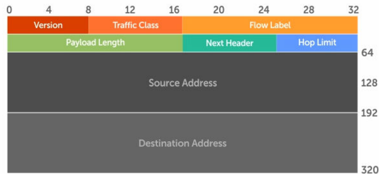
Figure 53. IPv6 Header Fields
